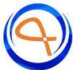
Min Bending Radius 5 ~ 6 Cable Diameter
