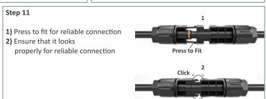
Note: Our Connectors are suitable for PV Solar cable of 2.5/4.0/6.0 mm diameter (As per EN 50618).
