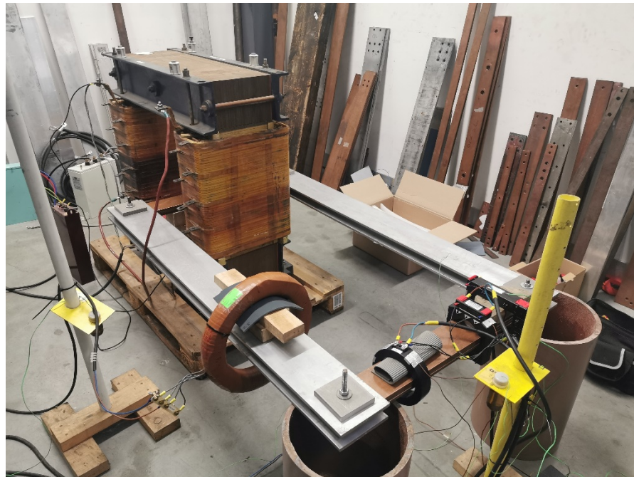
j) 3000/5A CT Photograph no. B26-20-AA-10E/04 Temperature-rise test
