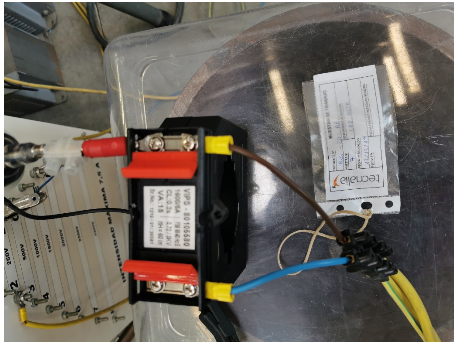
g) 1600/5A CT Photograph no. B26-20-AA-07E/03 Inter-turn overvoltage test
