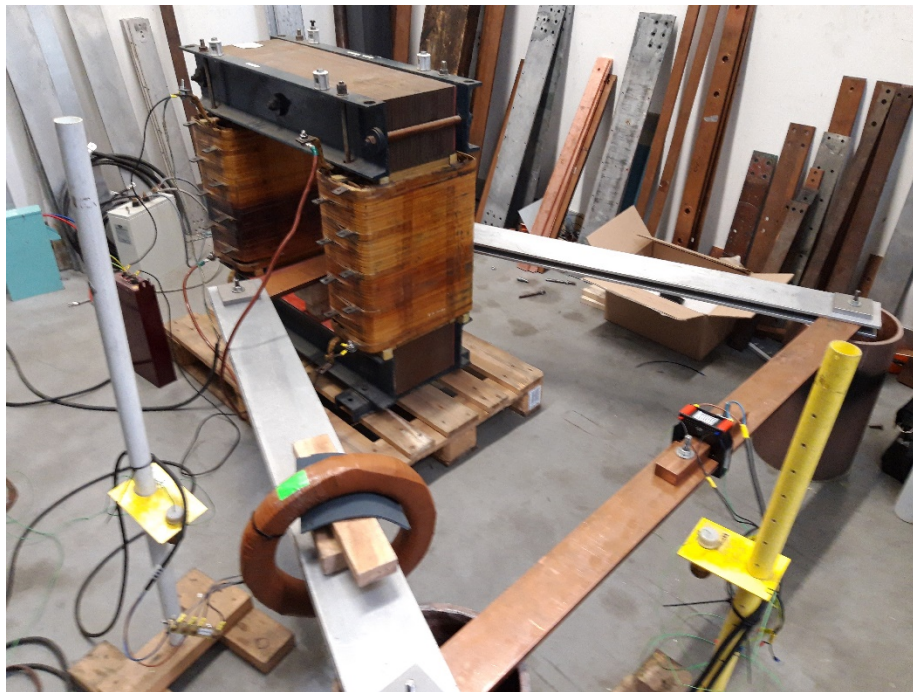
g) 1600/5A CT Photograph no. B26-20-AA-07/04 Temperature-rise test
