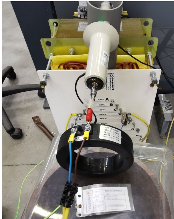
k) 3000/5A CT Photograph no. B26-20-AA-11E/03 Inter-turn overvoltage test
