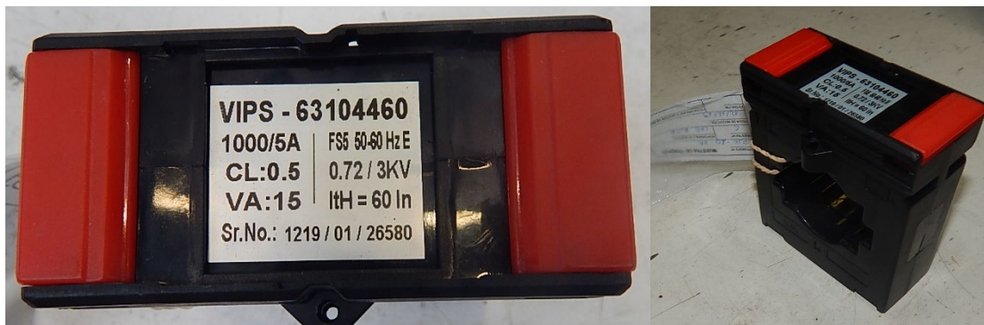
f) 1000/5A CT Photograph no. B26-20-AA-06E/06 After short-time current tests
