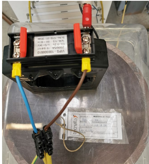
h) 2500/5A CT Photograph no. B26-20-AA-08E/03 Inter-turn overvoltage test
