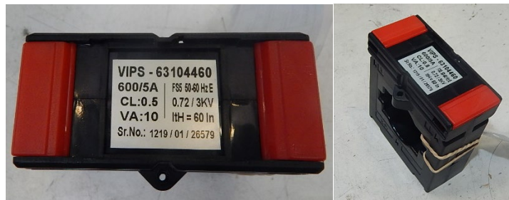
e) 600/5A CT Photograph no. B26-20-AA-05E/06 After short-time current tests
