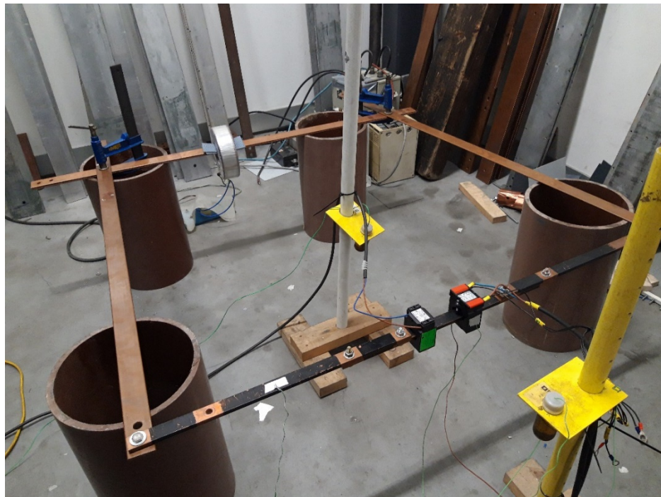
c) 300/5A CT Photograph no. B26-20-AA-03E/04 Temperature-rise test
