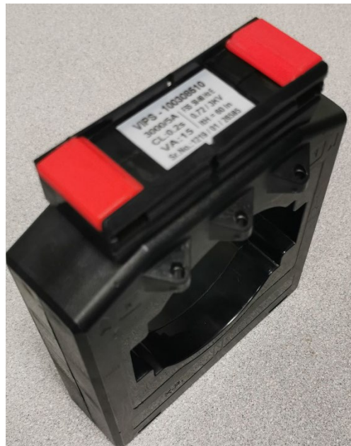
i) 3000/5A CT Photograph no. B26-20-AA-09E/06 After short-time current tests
