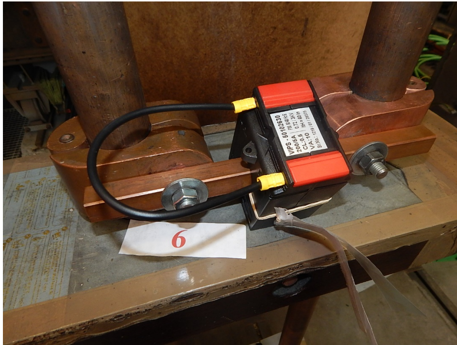
b) 200/5A CT Photograph no. B26-20-AA-02E/05 Short-time current tests
