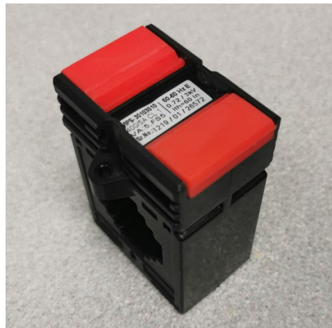
d) 400/5A CT Photograph no. B26-20-AA-04E/06 After short-time current tests
