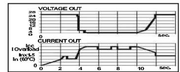
The output of the device is electrically protected against overload and short circuit. For the nominal voltage and nominal current at temperature condition, please see technical data. The device can supply at the nominal Current without switching off. As the overload increases, the output voltage is reduced until zero.
